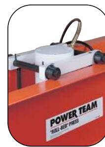
Cylinder is easily moved across width of upper bolster.
